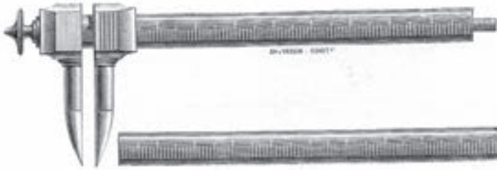
Fig. 9. Sliding aesthesiometer with ivory points created by the instrument maker Charles Verdin (1890, p. 43).
